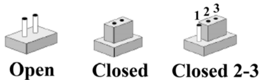
Figure 4 : Jumper Setting Illustrating
