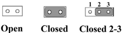
Figure 5 : Jumper Schematic Setting Illustrating
